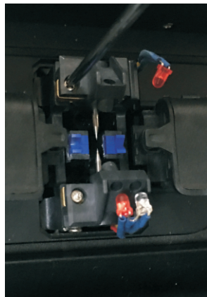
5.Screw out the screws with a screwdriver
