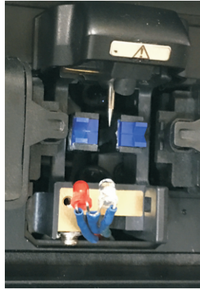
11. Close the electrode cap. Replace the other electrode by the same way
