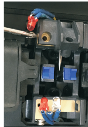
9 .Push the latch and install the screw
