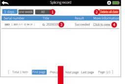
When save image is on, The system automatically saves the splicing records and images of each splice. The system can store 1000 splicing records and images internally.
