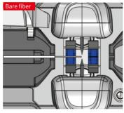
When [Endface Inspection] is on the,The fusion splicer will automatically check the fiber for damage and dust dust particles. If the following conditions are detected in the fiber, Please remove the fiber and re-prepare it.
